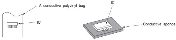
Fig. 1 Conductive container
